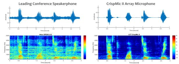
Side-by-side comparison in voice waveforms and spectrograms when recording at a distance.
